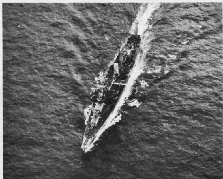
Oldest U. S. heavies, Pensacolas are the only ones which mount ten 8-in. guns. View from above shows this heavy armament arranged in four twin and triple turrets. Note tall stacks and lofty tripod foremast.
